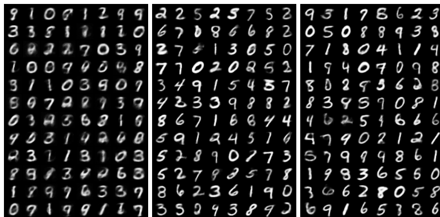
FIGURE B.11: Samples after iterations 0, 40, and 90 epochs on VAE with convolutional layers for MNIST dataset
